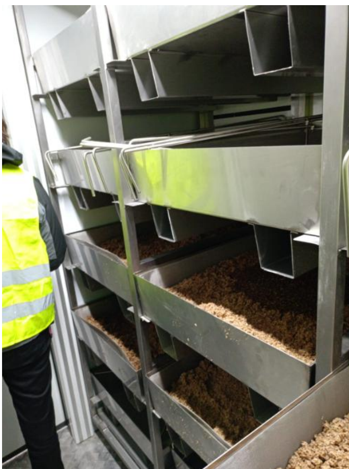
Figure 8. fattening boxes in stainless steel larger capacity than plastic boxes
