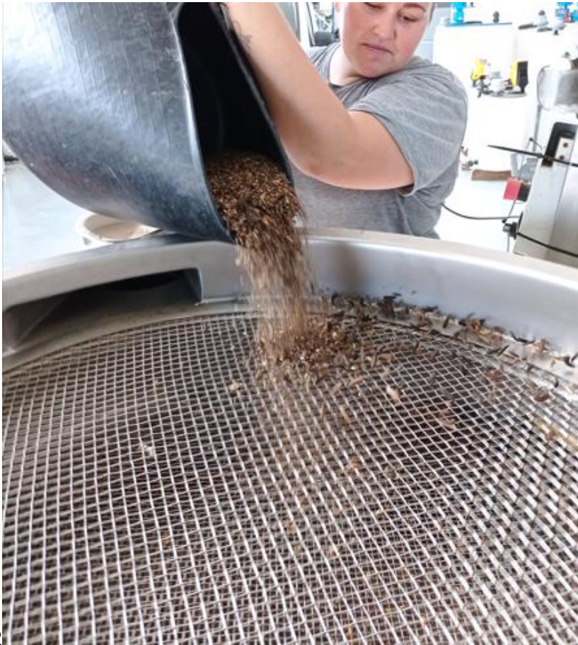
Figure 11. mechanical sieving to separate larvae from frass
