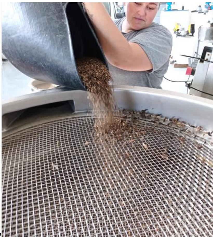
Figure 11. mechanical sieving to separate larvae from frass
